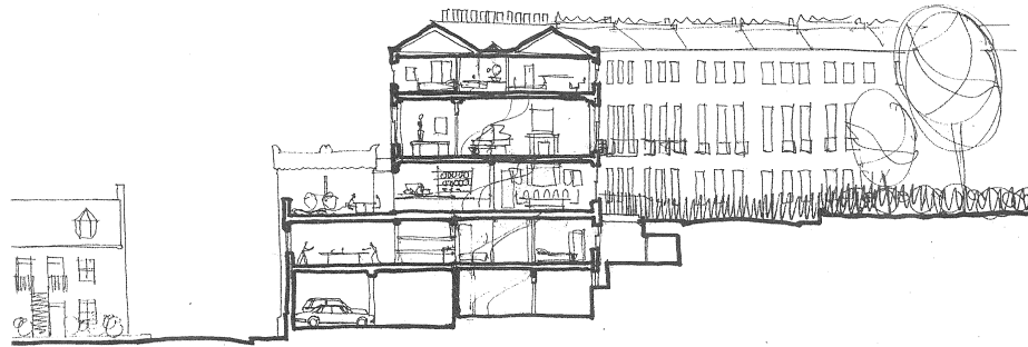
sketch section through 5-storey townhouse with terrace garden and garage
